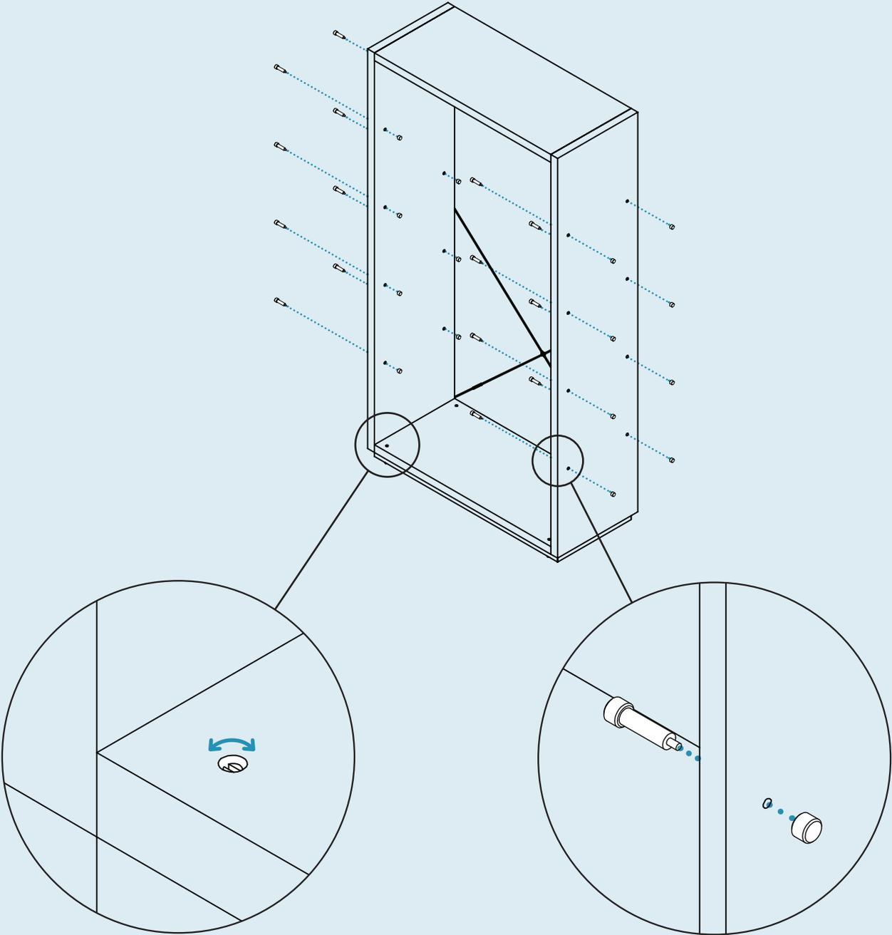
Turn to adjust the feet height to level the case.
