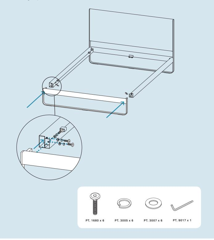
INSTALLING THE CENTER LEG.
